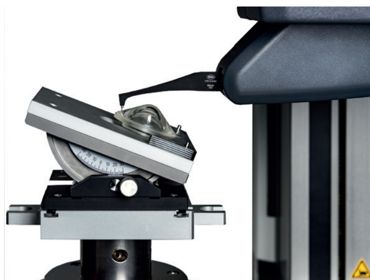
Measurement of steep aspheres with stitching, step 1: measuring left flank of lens
